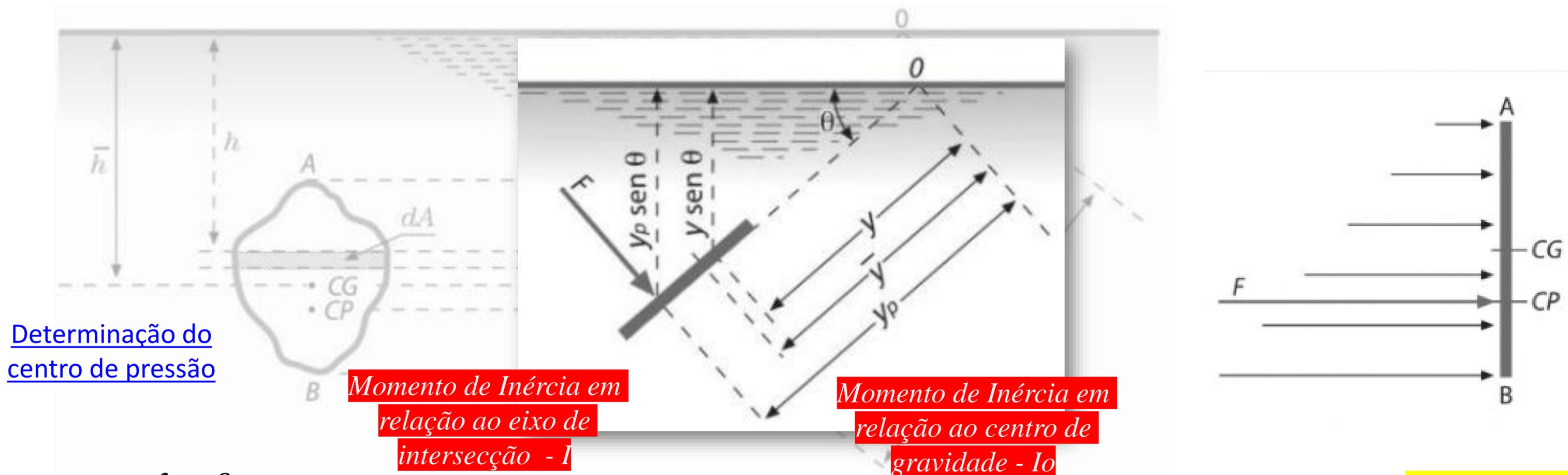
$$y_p = \frac{\int_A y^2 \times dA}{\bar{y} \times A} \quad \int_A y^2 \times dA = I \quad \rightarrow \quad y_p = \frac{I}{\bar{y} \times A} \quad I = I_o + A \times \bar{y}^2 \quad \rightarrow \quad y_p = \frac{I_o + A \times \bar{y}^2}{\bar{y} \times A} \quad y_p = \bar{y} + \frac{I_o}{\bar{y} \times A}$$
