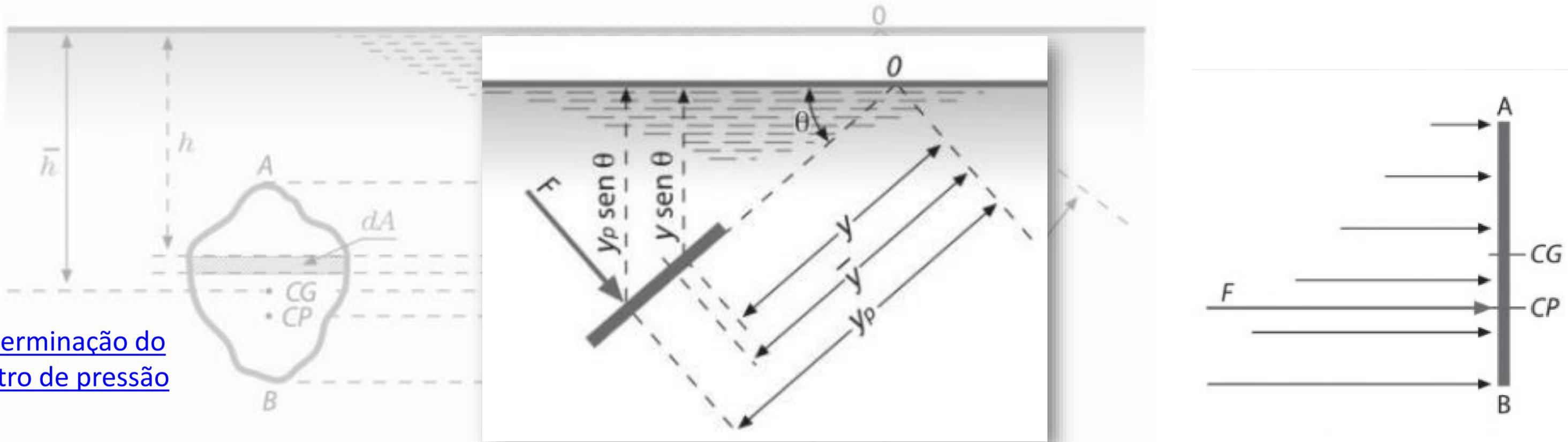
$$\gamma \times \text{sen}\theta \times \bar{y} \times A \times y_p = \gamma \times \text{sen}\theta \times \int_A y^2 \times dA \rightarrow y_p = \frac{\gamma \times \text{sen}\theta \times \int_A y^2 \times dA}{\gamma \times \text{sen}\theta \times \bar{y} \times A} \rightarrow y_p = \frac{\int_A y^2 \times dA}{\bar{y} \times A}$$
